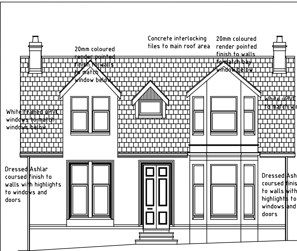
EXISTING WEST ELEVATION
